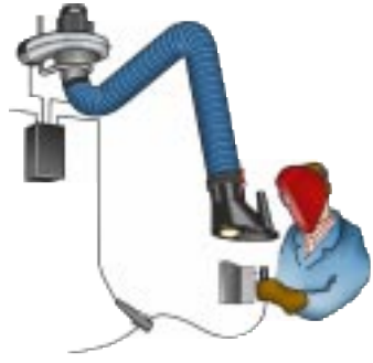
The extractor arm can be equipped with a spot light and an automatic start/stop control for the fan.
